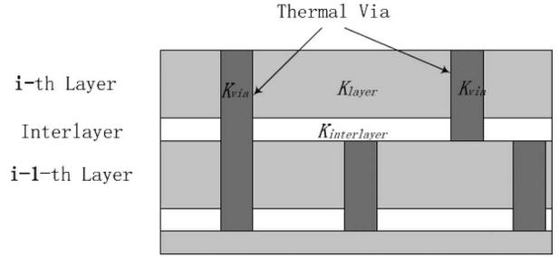
Fig. 3. T-via density and thermal conductivity.
