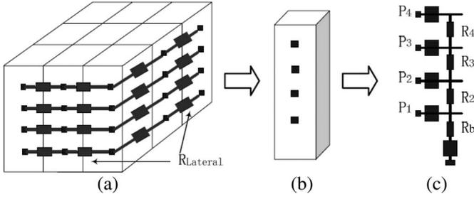
Fig. 2. Compact resistive thermal model. (a) Tile stack array. (b) Single tile stack. (c) Resistance.
