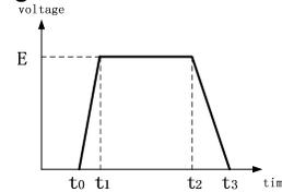
Figure 2. Ramp signal waveform
