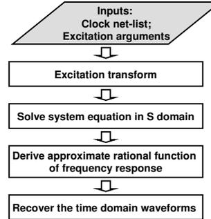
Figure 1. Flow chart of CSAV
