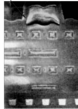
Figure 9. A realistic vertical cross section of IC interconnect. We see that conductors on layers 1–5 are trapezoidal, and there is a conformal dielectric on top of the top layer metal (passivation). (SEM photograph courtesy of IBM Corp. © Copyright IBM Corp. 1994, 1996.)
