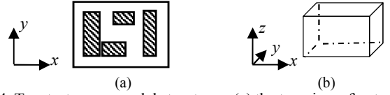
Fig. 4: Two test macromodel structures. (a) the top view of a structure containing 4 conductors. (b) the 3-D view of an empty half-cube.
